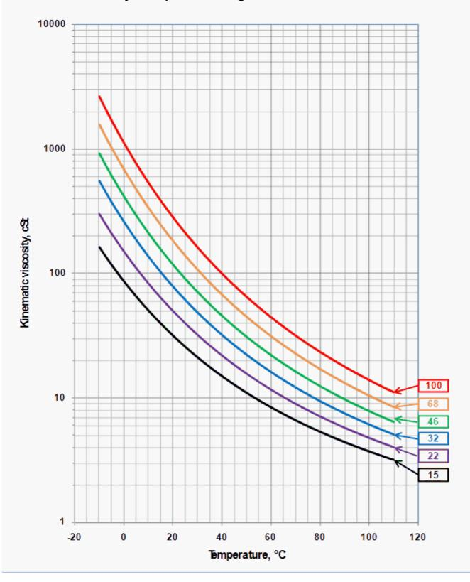
Viscosity - Temperature Diagram for Shell Tellus S2 V
